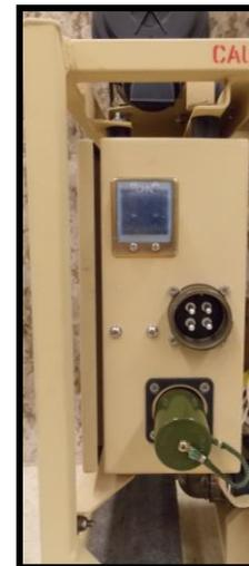
A simplified control box allows the generator to be placed in auto mode with the flip of a switch. Output voltage and loads are monitored on the analog meters. An engine hour meter is located on the front panel along with LEDs that provide status and fault indications. A digital data connector and battle short switch are located on one side panel and the main circuit breaker. A NATO slave for electric starting and a generator output connector to loads are located on the other side panel.
